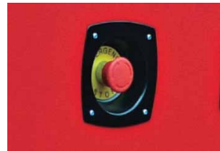
Emergency Stop Button Easy reachable on outside
